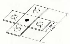
Fig. 1 — Cross-tension specimen
