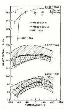
Fig. 16 — Impact shear strength of VAN-80 and SAE 1008 steel spot welds
