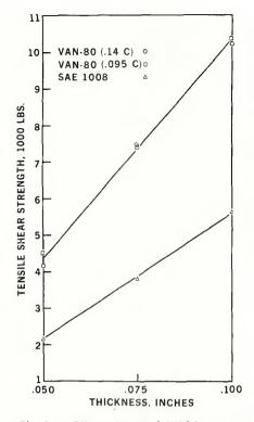
Fig. 9 — Effect of material thickness on the tensile shear strength of spot welds in VAN-80 and SAE 1008 steel
