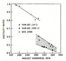
Fig. 15 — Dependence of ductility ratio on weld nugget hardness
