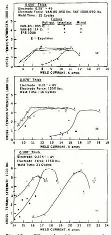
Fig. 13 — Effect of weld current on the cross-tension strength of spot welds in VAN-80 and SAE 1008 steels
