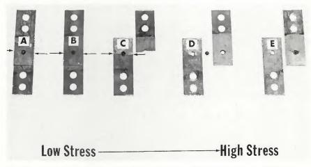
Fig. 19 — Fatigue failures. Arrows indicate failure locations on low stress specimens
