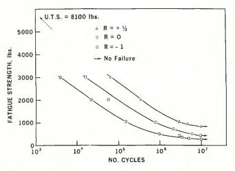
Fig. 17 — Fatigue strength of spot welds in 0.082 in. thick VAN-80(.14C)
